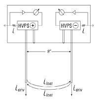
Simco-lon design for maintaining stable ion current flow despite fluctuating environmental conditions, point erosion and point "aglomeration" (+HVPS Alarm - level set at factory).
