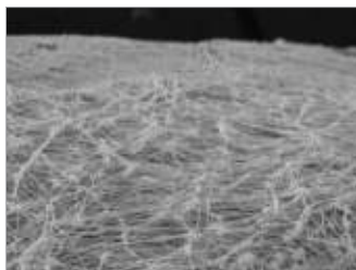
Resilient ePTFE Filtration Technology media at fold tip @ 10,000x magnification.
